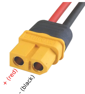
Figure 11.4: Charger input pinout – Amass XT60 female (controller side)
